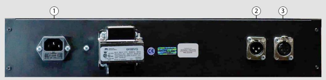
(1) AC Power Connector / Fuse Holder - Connect a standard, detachable IEC power cable (supplied) here. If fuse replacement is required, use only a 125 mA time delay (slow blow) fuse for operation at 115 V, or a 63 mA time delay (slow blow) fuse for operation at 230 V.
